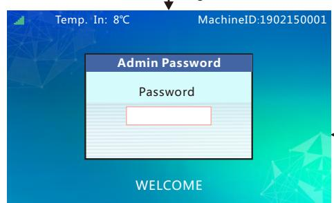
Press the digital keyboard to enter the password, the initial password is "000000"
